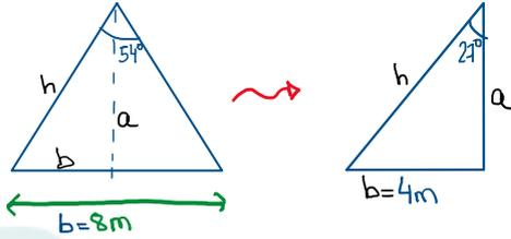
a)  $\text{sen } \alpha = \frac{\text{c.op}}{h} \rightarrow \text{sen } 27^\circ = \frac{4}{h} \rightarrow h = \frac{4}{\text{sen } 27^\circ} = 8,81 \text{ m.}$
