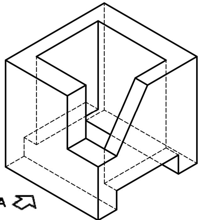
A A reference symbol consisting of the letter 'A' above a small triangle, indicating the view used for the elevation.
